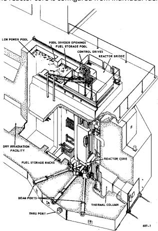
The reactor core is configured from individual fuel elements placed in a core grid box 26 feet
